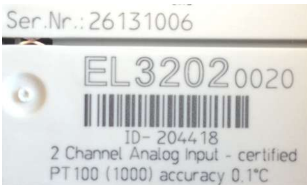
Fig. 4: EL3202-0020 with batch numbers 26131006 and unique ID-number 204418
