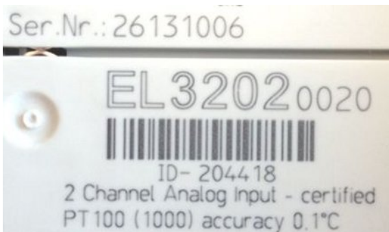
Fig. 4: EL3202-0020 with serial/ batch number 26131006 and unique ID-number 204418
