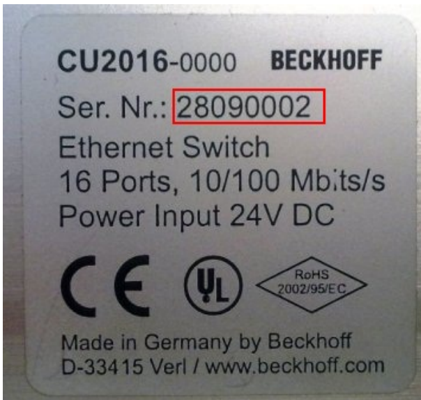
Fig. 3: CU2016 switch with batch number
